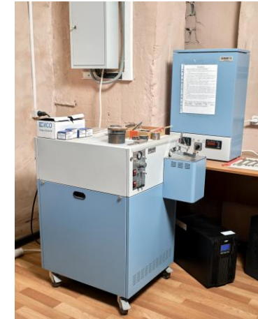
• DFS-500 spectrometer optiko- issue for the analysis of metals
